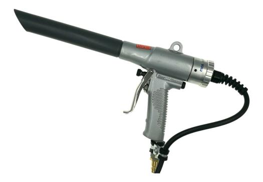
The AG-02 antistatic gun is a transvector compressed air gun that removes static charge. The ionization pin is of the "shockless" type - without danger when touched. In addition, the pin is protected in a robust gun body. This allows the air flow to ionize when the trigger is pressed, thereby eliminating electrostatic charges that occur on product surfaces.
