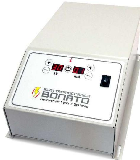
**ECG50** charge generator creates an adjustable high voltage between 5 to 50 KV and an also adjustable current between 0 and 2,5 mA. Its controls are very intuitive and thus easy to be used by the operator. Besides it can be remotely controlled by means of the remote control analogical function. It can have positive or negative charge on request and from 1 to 4 high voltage outputs.
