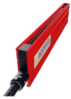
CBR-LP-15 low profile electrostatically charging bars are designed to make a material adhere to a surface or two materials between them. These charging bars are connected to a generator, which creates (positive or negative) ions on bar's pointed edges by means of high voltage. Thus the material, passing through the bar and a reference mass, is pushed towards the mass itself, creating a temporary adhesion.
